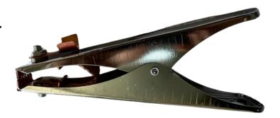
Heavy-duty spring clamp for returning welding current to the workpiece. Steel body with copper/brass contact inserts for low resistance. Serrated jaws and strong spring for secure grip on plate, angle, or pipe.
