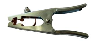
Heavy-duty reinforced body ground clamp for high current return. Wide jaws with copper inserts and a high-tension spring deliver low resistance and stable clamping on tables, plates, or pipes. Bolt post for cable lug.
